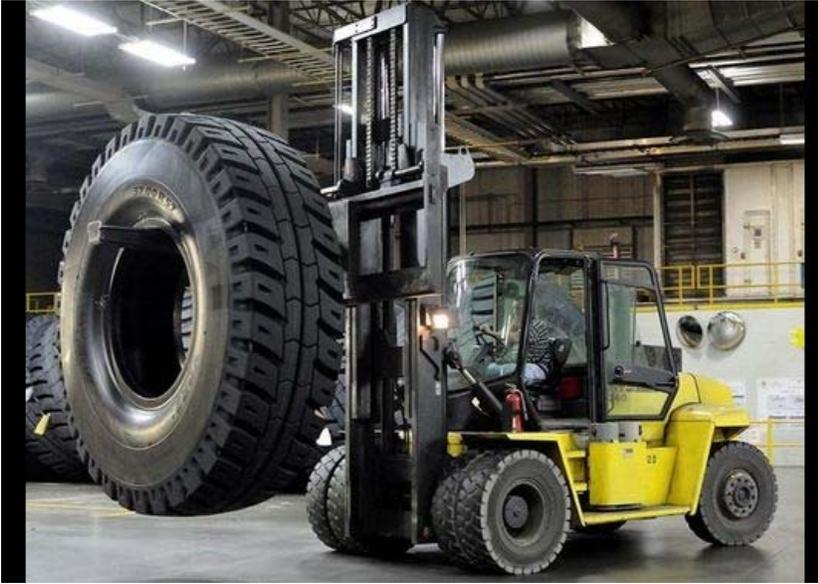
**Large fork lifts are required to move Michelin's massive Earthmover tires after being produced at the company's production plant in Lexington, SC.** (Photo: Michelin North America)
