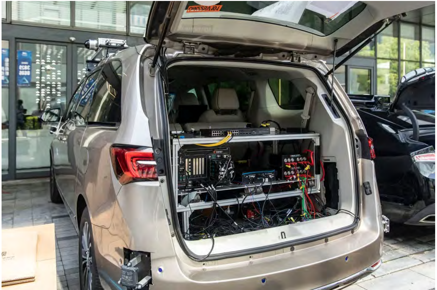
Data collection equipment for autonomous driving in a test van outside the Kunyi Electronics Technology plant in Shanghai. Qilai Shen for The New York Times
